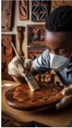
Applying Lacquer to a wood carving to give it a glossy finish
