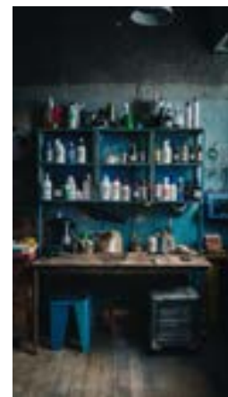
Figure 79: Inadequate/ ineffective storage of chemical products in a studio.
