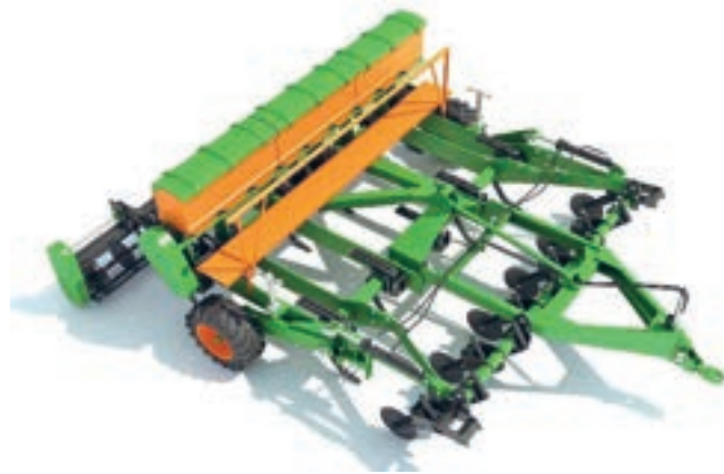
Fig. 3 wk8: Picture of a seed harrow combined with a seed drill
