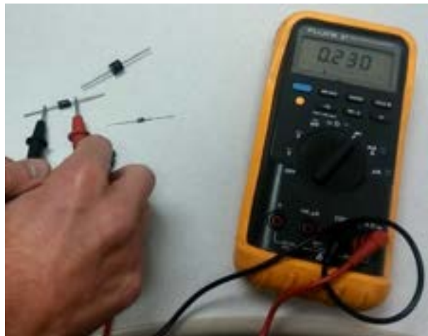
Fig. 6.5: A technician using a multimeter to test a diode.
