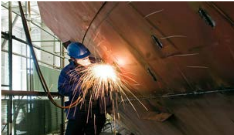
Fig. 5.20: Gas welding in shipbuilding and marine industries.
