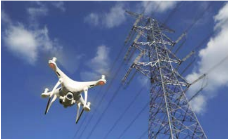
Figure 20: Drone for inspection
