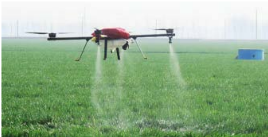
Figure 21: Agric spraying drone
