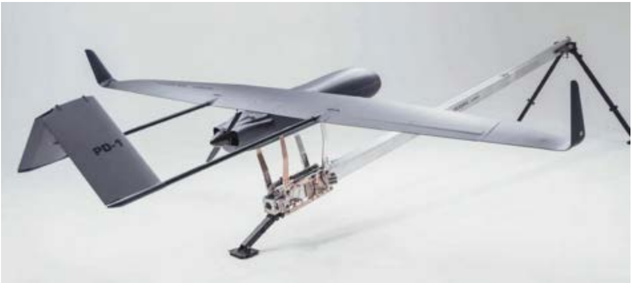
Figure 18: UAV pneumatic catapult- launch
