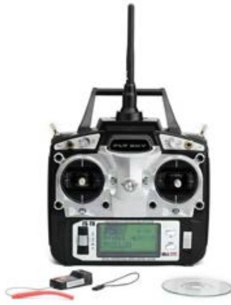
Figure 15: Radio transmitter and receiver
