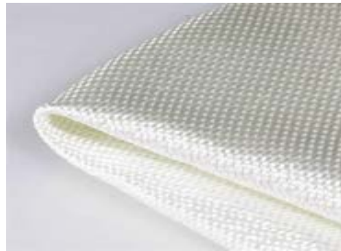
Figure 14: Fibreglass material used in electrical insulation.
