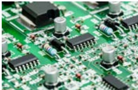
Figure 10: Electronic components mounted on a printed circuit board.
