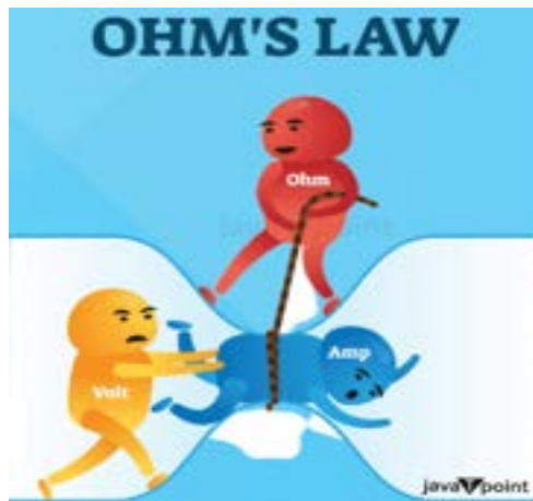
Figure 17: Voltage pushes the current through the conductor while the resistance “resist” the flow of current through the conductor.
