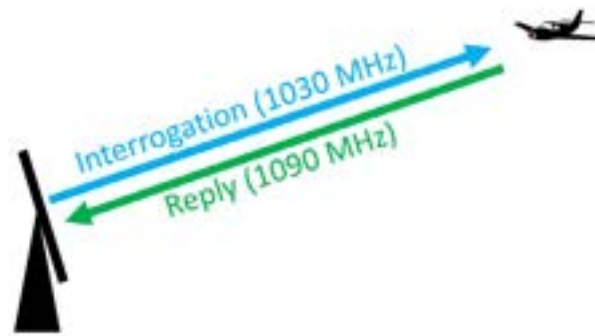
Figure 34: Secondary surveillance radar operation.
