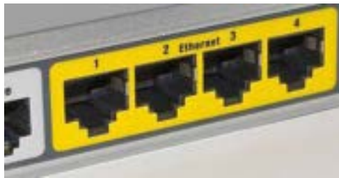
Figure 20.9: Rear of a router
