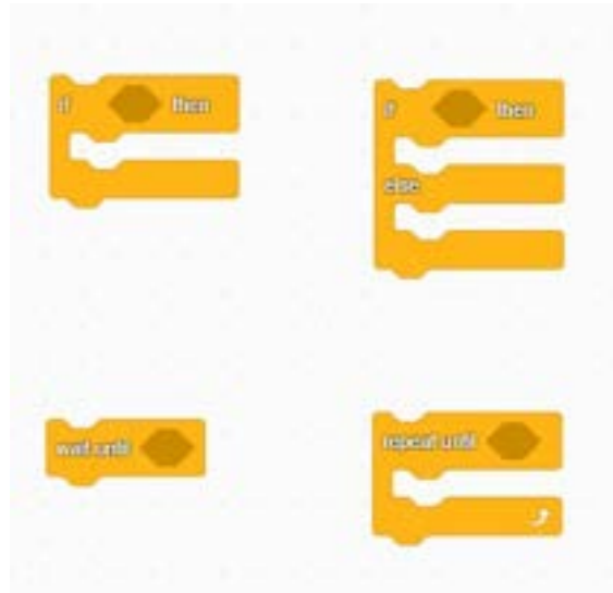
Fig. 21.4: Examples of Control Blocks in the LEGO Education SPIKE app that are used to implement decisions
