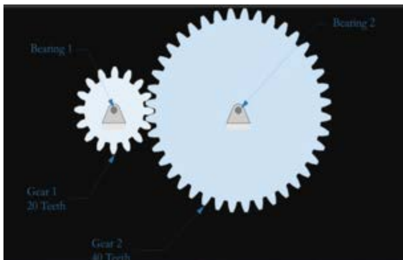
Fig. 19.4: Diagram showing Gear 1 with 20 teeth and Gear 2 with 40 teeth
