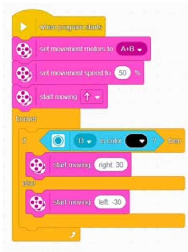
Fig. 24.2: Block program showing a line following robot which uses nested blocks
