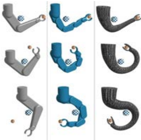
Fig. 18.2: Robots with rigid structures and structures that lack rigidity (Charbel Dalely, Tawk Gursel Alici, Comparison of the proposed robotic arm system and related designs. | download scientific diagram 2021)
