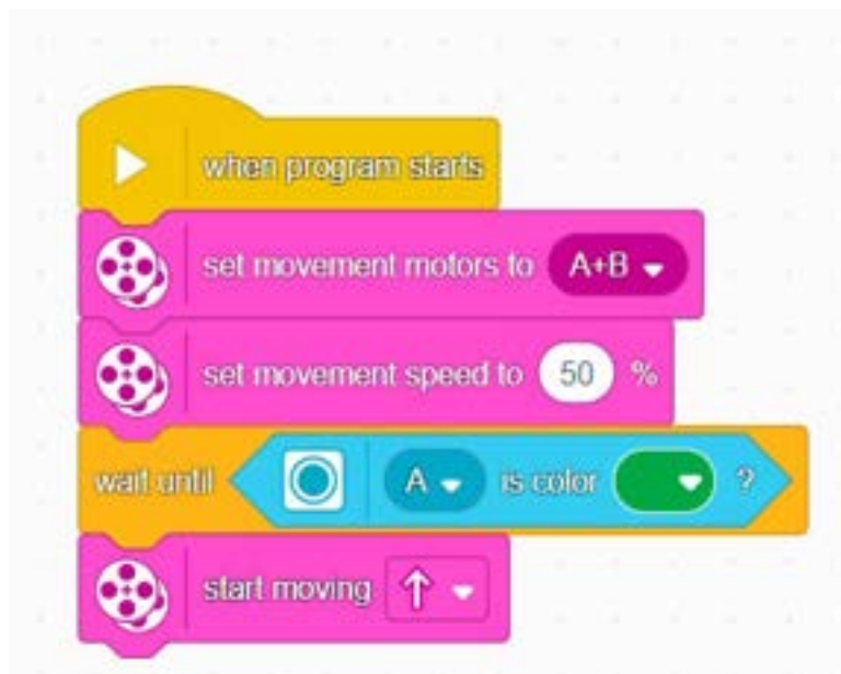
Fig. 21.11: Block programme which implements the flowchart using a wait-until block.
