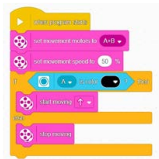
Fig. 21.9: Block programme which implements the flowchart using an if then else block.
