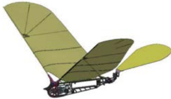
Fig. 19.9: Flapping Wing Aerial Robot (Zhong & Xu, Power modelling and experiment study of large flapping-wing flying robot during forward flight 2022)
