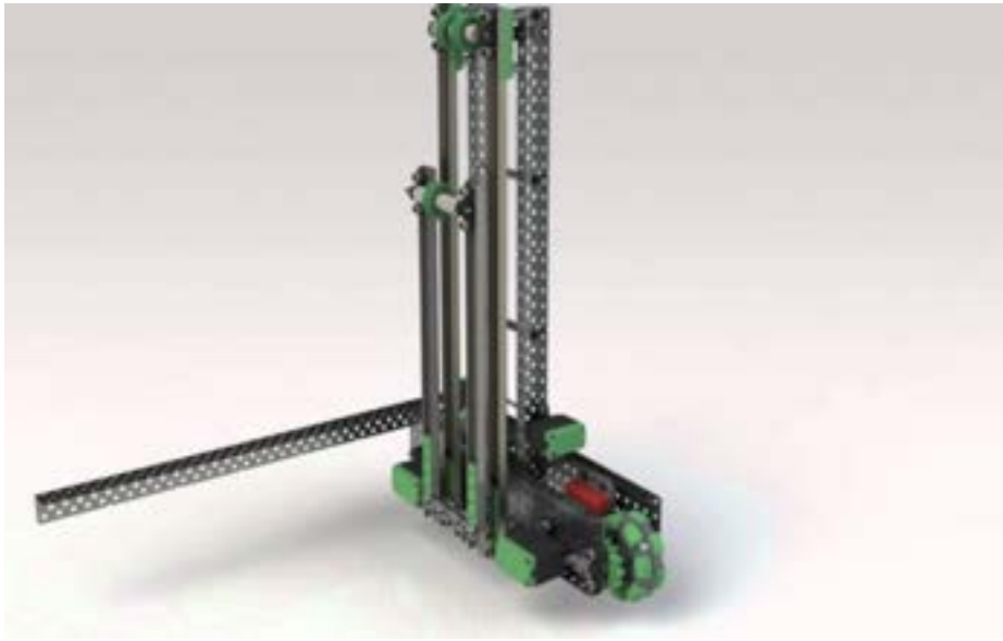
Fig. 19.11: Lifting Mechanism Robot (254 VEX talk: Episode 3 - an overview of lifts 2012)
