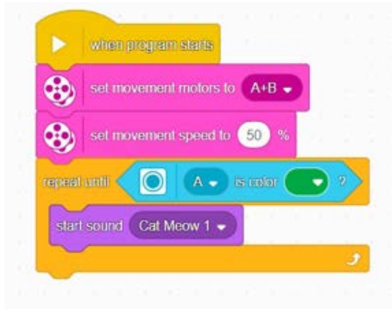
Fig. 21.14: Block programme which implements the flowchart using a repeat-until block.
