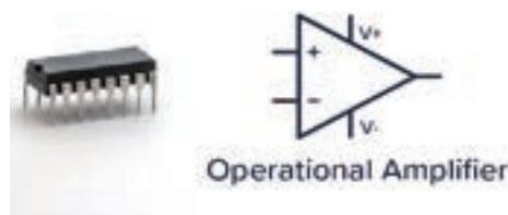
Fig 9.6: An Integrated Circuit and a symbol of an IC
