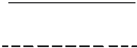
Fig. 5.4: Solid and Dashed Lines used in Loop Diagrams
