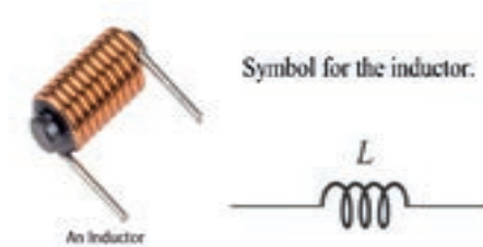
Fig 9.3: An actual Inductor and the symbol for an inductor
