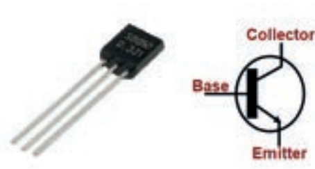
Fig. 9.5: A Transistor and a symbol of a transistor
