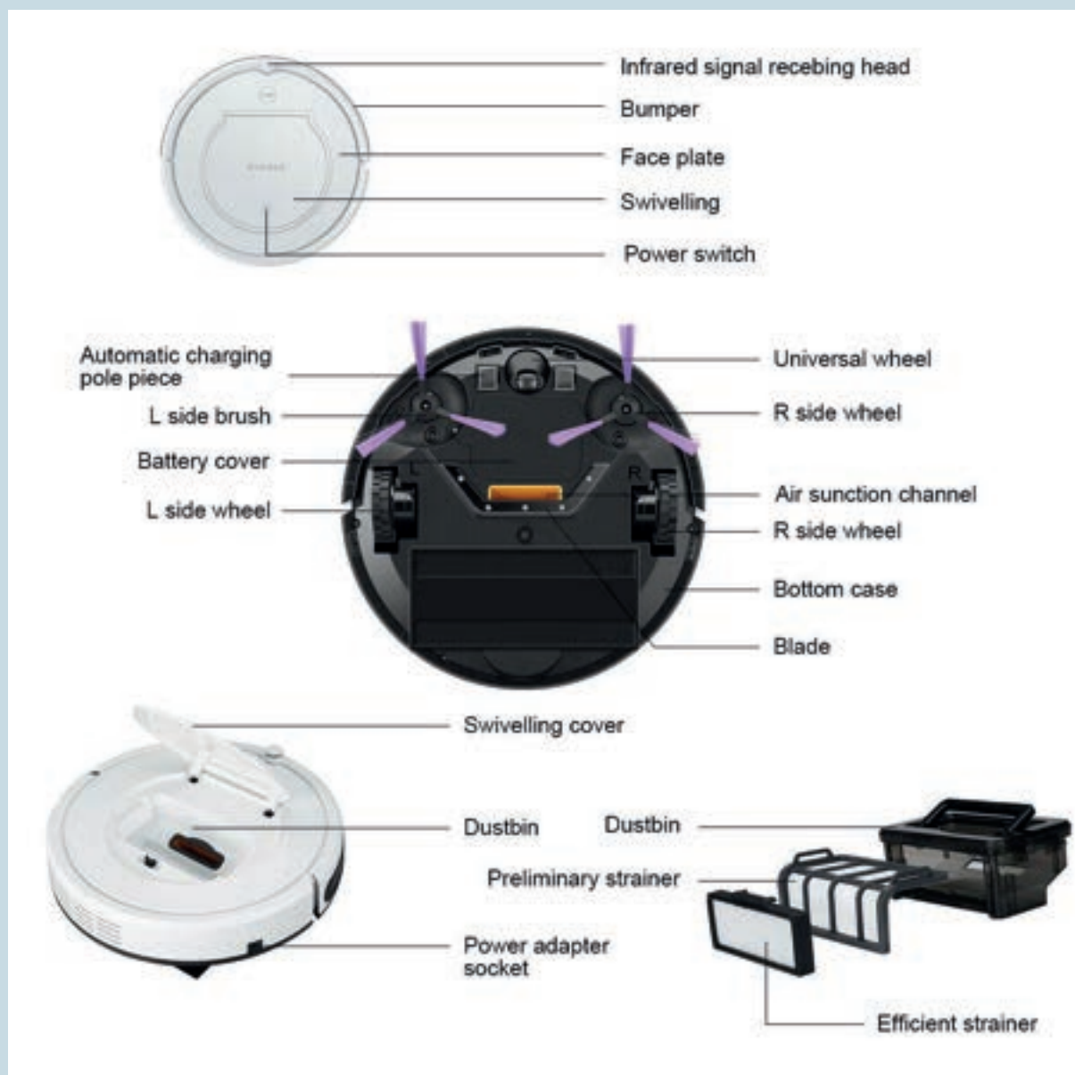
Fig. 3.2: Parts of a Robotic Vacuum Cleaner
