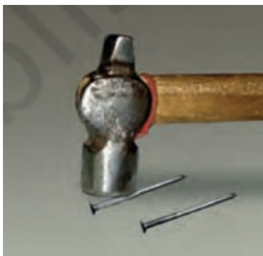
Fig. 2.4: Testing malleability of metal
