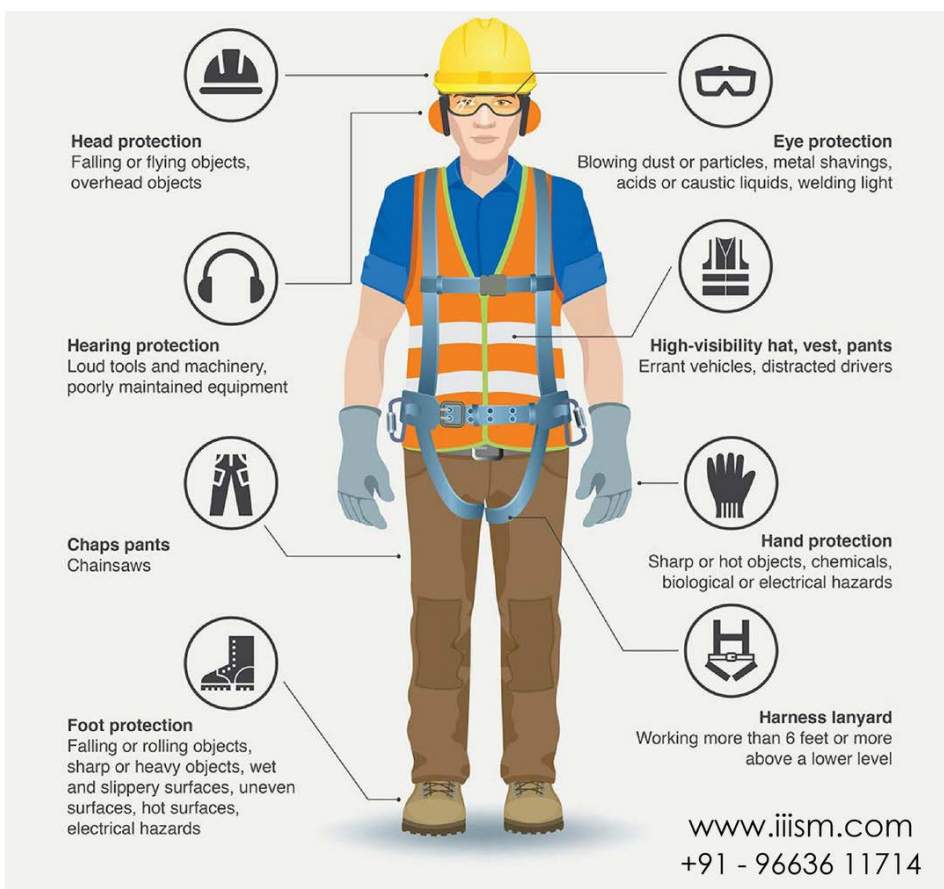
Fig. 1.5.1: Personal Protective Equipment and Demonstration of How to Use Them
