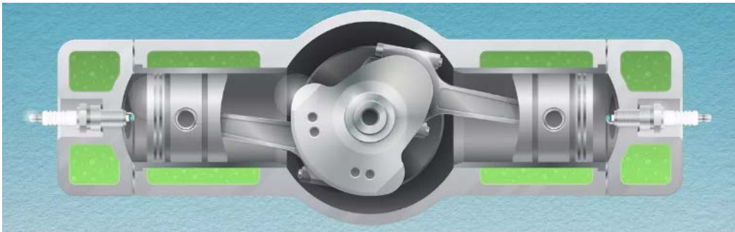
Fig. 1.2.8: Flat engine design (source: www.cars.com )
