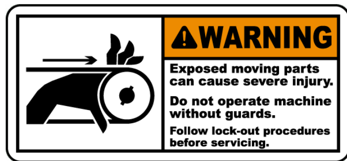
Fig. 1.1.8: Warning Safety Label: Exposed moving parts can cause severe injury.
