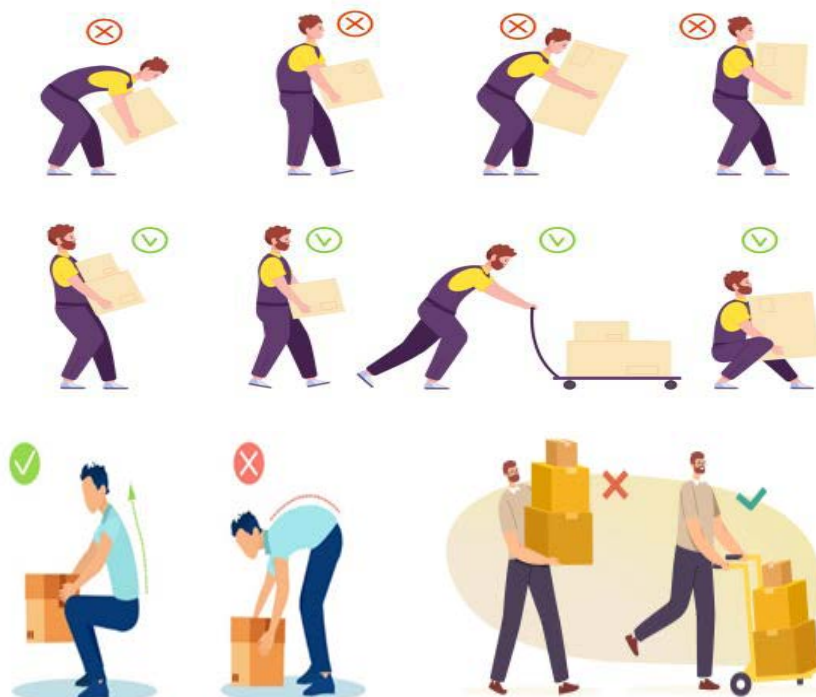
Fig 1.5.5: Proper Manual Lifting Techniques
