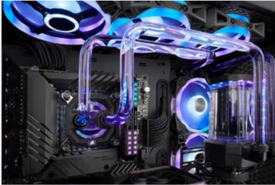
Figure 2.38 Gaming desktop having a custom liquid cooling system on the CPU.
