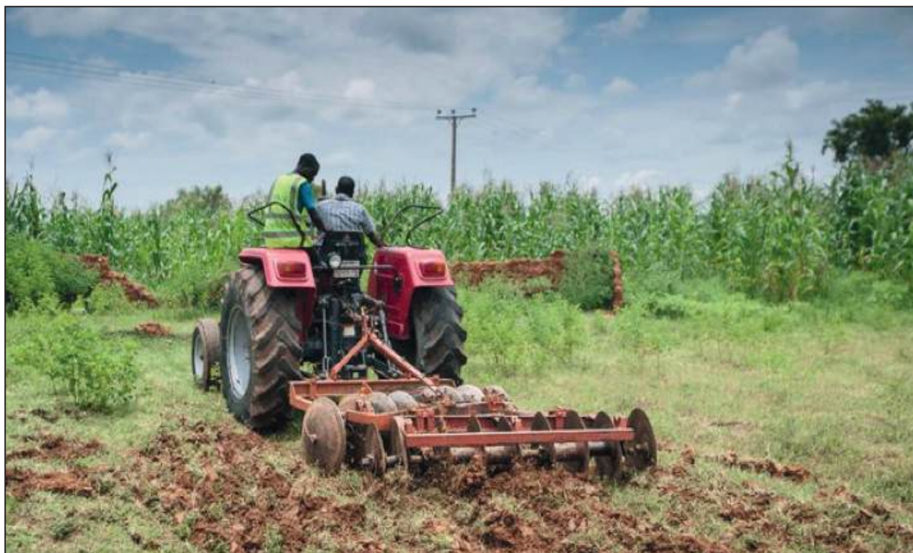
Fig. 11.2: Farmer working with disc plough mounted on a tractor
