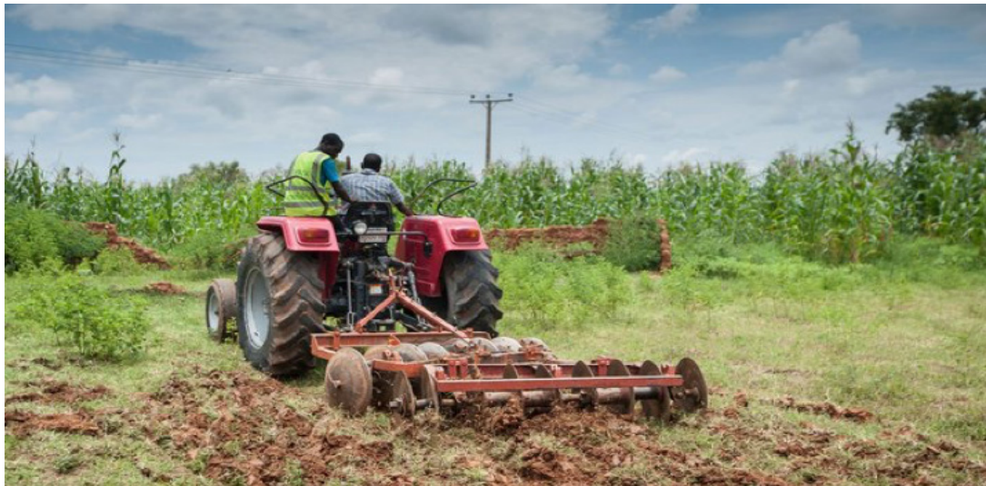
Fig. 6.2: Farmer working with disc plough mounted on a tractor.
