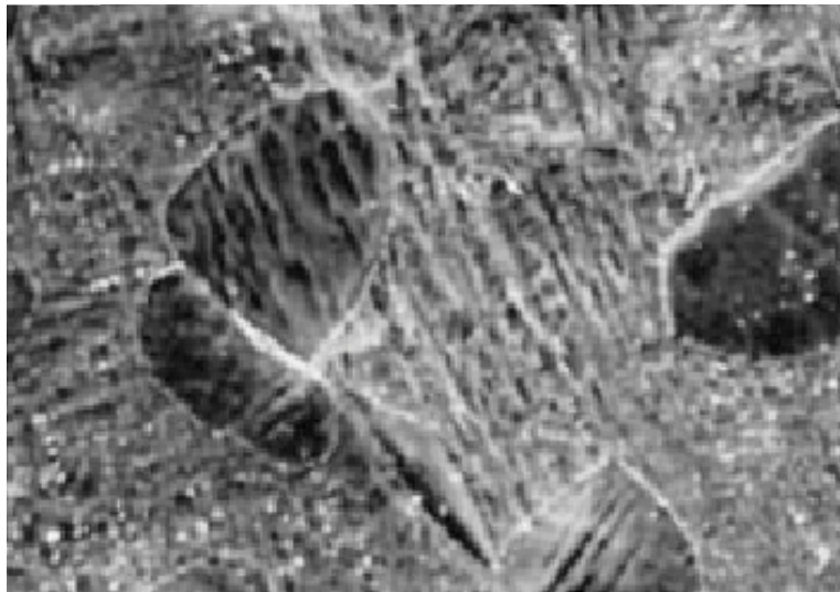
Fig. 1.12: Titanium alloy (Ti-6Al-4V) at 5 \mu\text{m}
