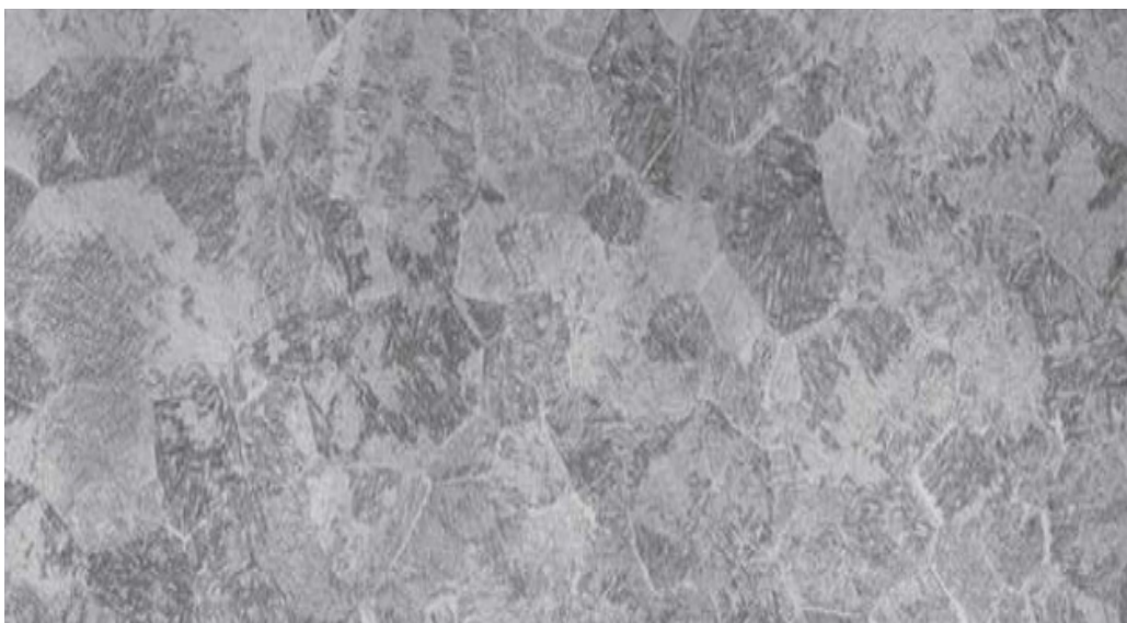
Fig. 1.13: Macrostructure of Titanium alloy (Ti-6Al-4V) at a resolution of 1 mm
