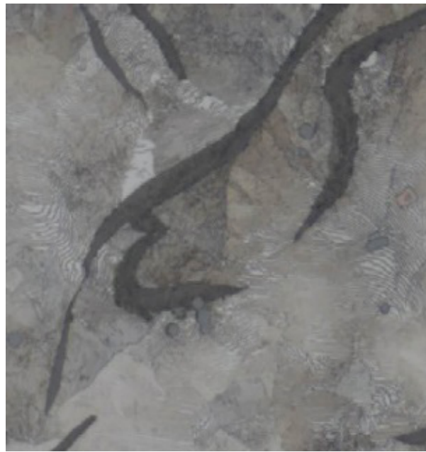
Fig. 1.10 Cast iron ( Pearlitic cast iron ) at 25 \mu\text{m}
