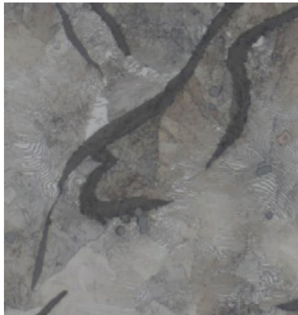
Fig. 1.10 Cast iron ( Pearlitic cast iron ) at 25 \mu\text{m}
