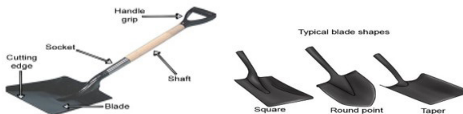
Fig. 2.9: A diagram of a spade. Heads of spade and shovel (middle)
