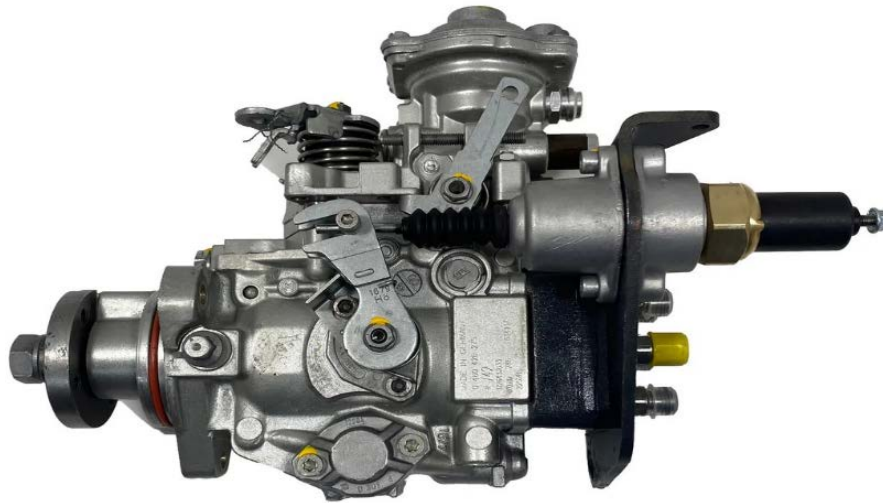
Fig. 2.2.11: A mechanical diesel injection pump (source: goldfarbinc.com)
