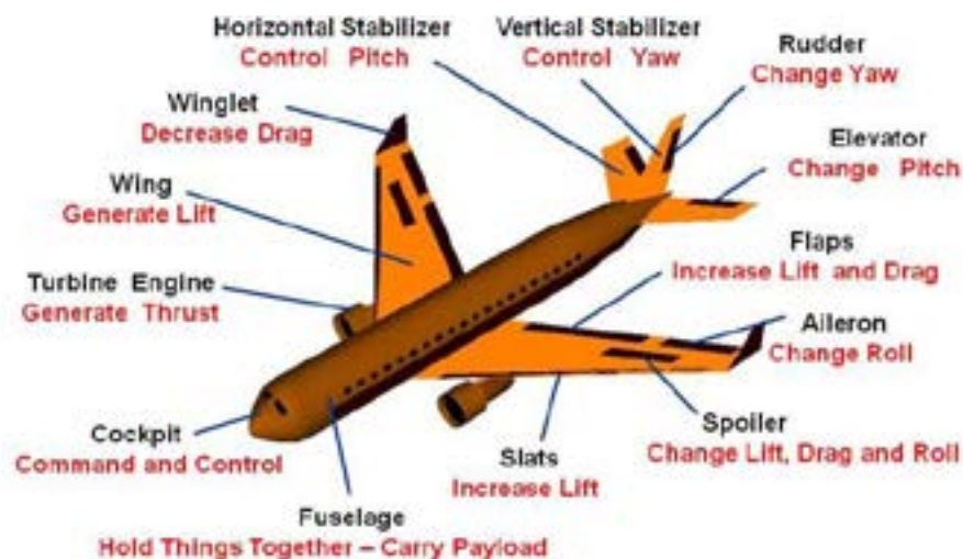
Figure 1.14 Parts of a fixed-wing aircraft
