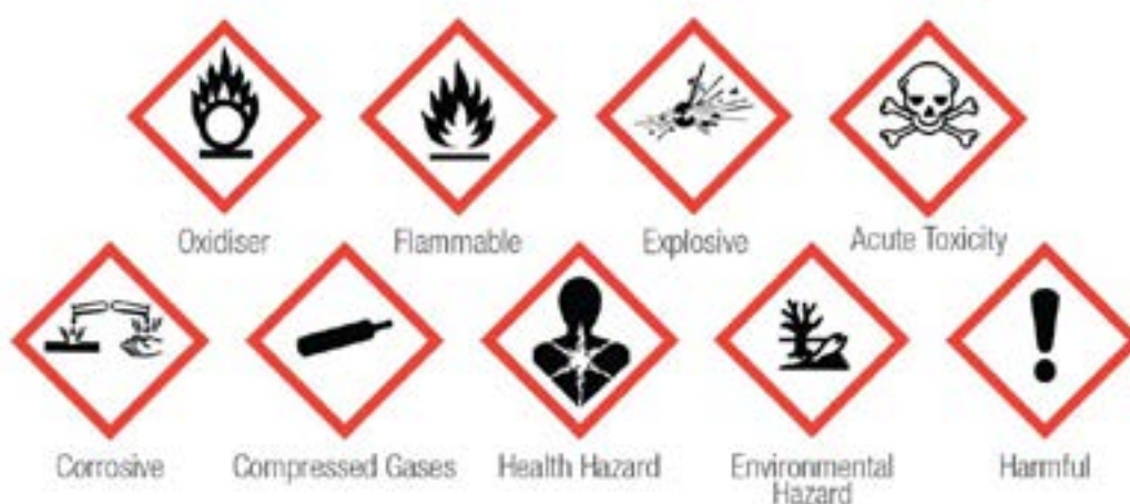
Fig. 2.2: Sample Safety Hazard Signs
