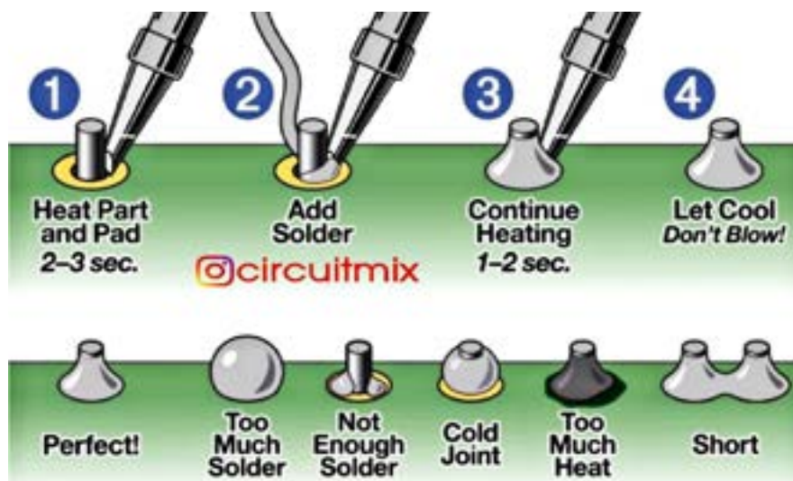
Fig. 3.30 An image showing the proper way to solder.
