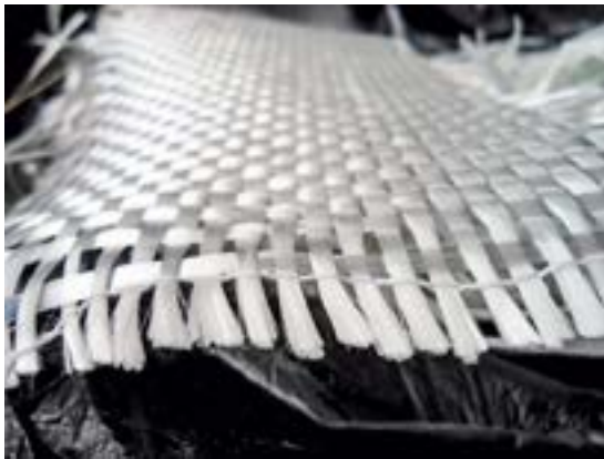
Fig 3.4. Fibreglass material is used in electrical insulation
