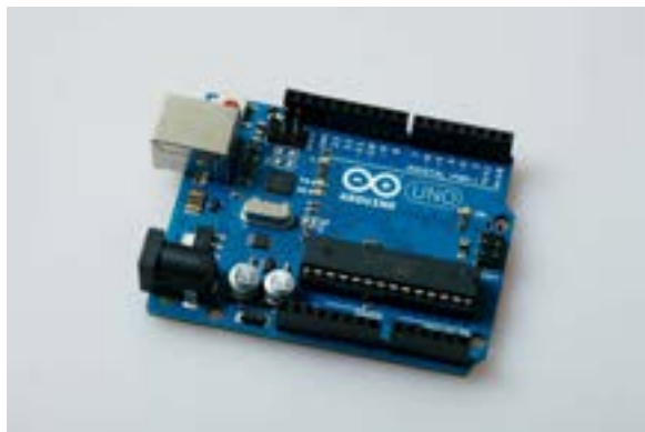
Fig. 3.16. Arduino microcontroller board based on the ATMEGA328p chip. Image ID: D7756M
