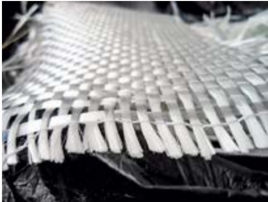
Fig 3.4. Fibreglass material is used in electrical insulation
