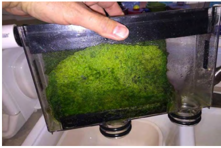
Figure 2.3: A algae scrubber
