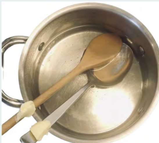
Fig 3.1 Different spoons with shea butter on the handle in hot water
