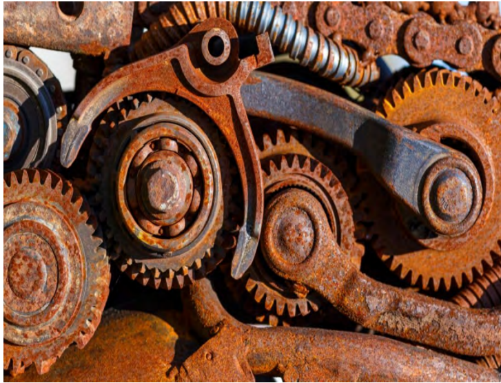
Figure 2.6: metal parts under going rusting
