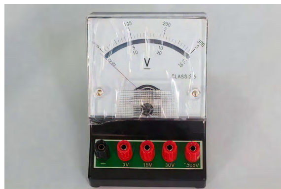
Fig. 1.5: An analogue voltmeter having negative zero error
