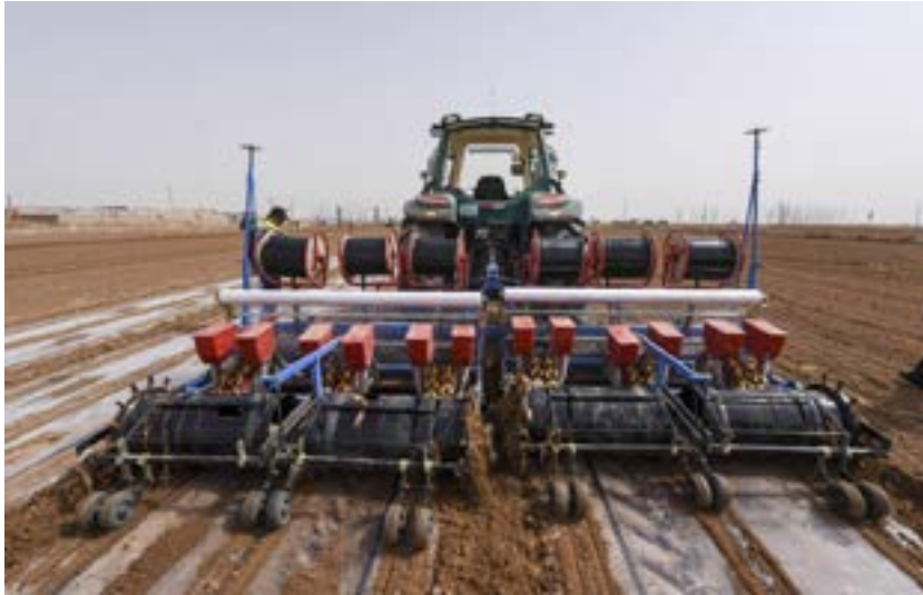
Fig. 2.2 A self-driving tractor sows cotton seeds in the field at Yaha Township of Kuqa County, northwest China's Xinjiang Uygur Autonomous Region, March 23, 2018. The smart tractor, with automatic navigation system, can do farm work itself including ploughing and seeding.
