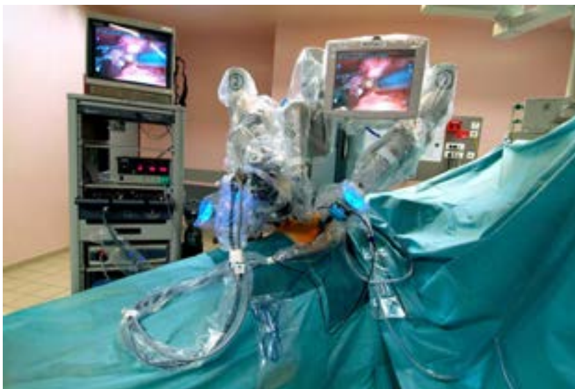
Fig. 2.1 Da Vinci robot surgeon performing keyhole (laparoscopic) surgery, a remote-controlled surgical system, developed and produced by the US company Intuitive Surgical.
