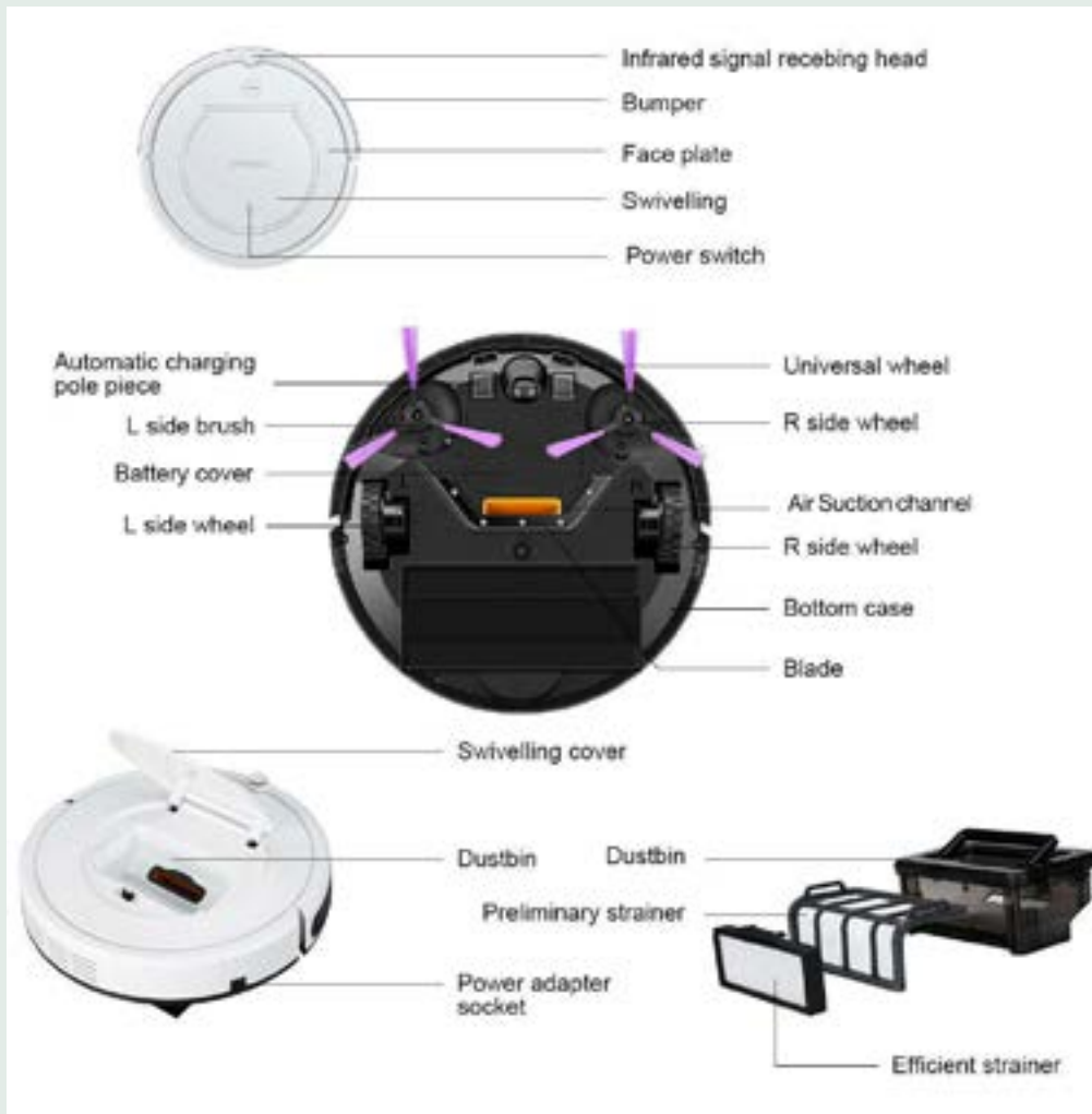
Fig. 2.4 Subsystems of a robotic vacuum cleaner ().
