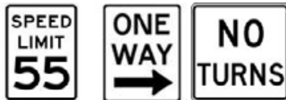
Fig. 2.12: Black and white signs provide motorists with regulations and laws governing use
