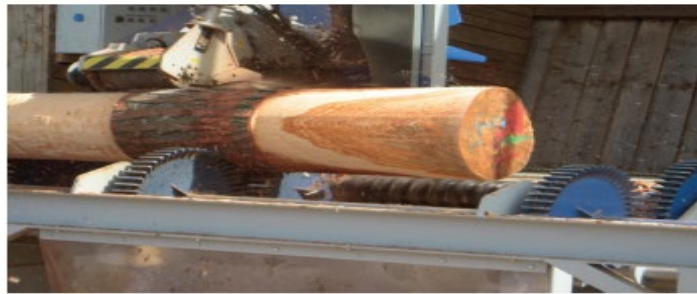
Fig.3.1.4: Process of debarking
