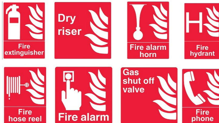
Fig. 3.2.17: Examples of fire safety signs
