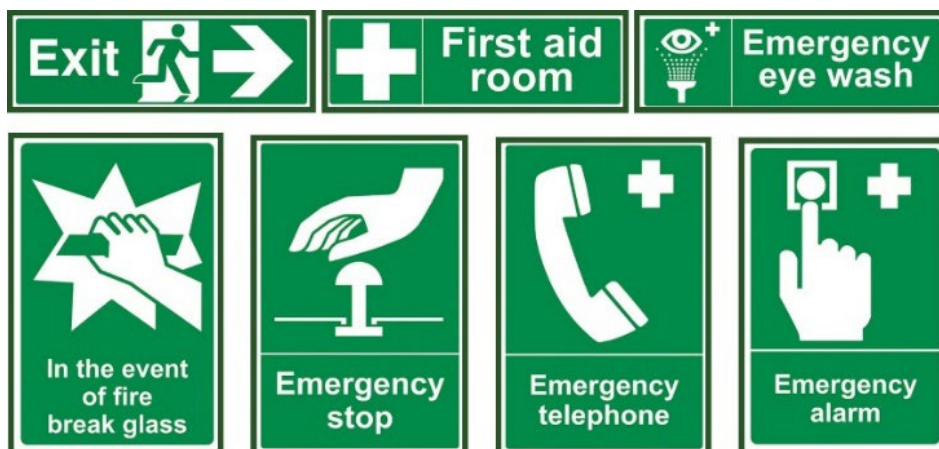
Fig. 3.2.16: Examples of emergency information signs
