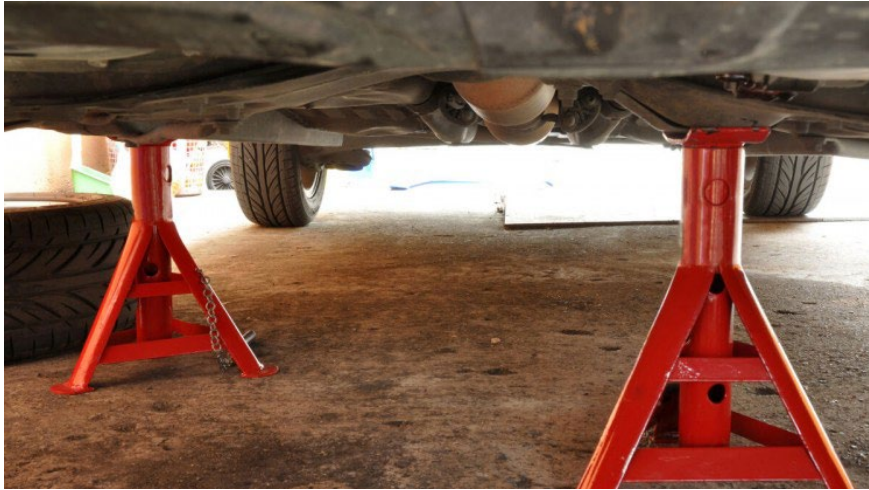
Fig. 3.2.4: Raised car supported on axle stands (Source: vehiclescene.com)
