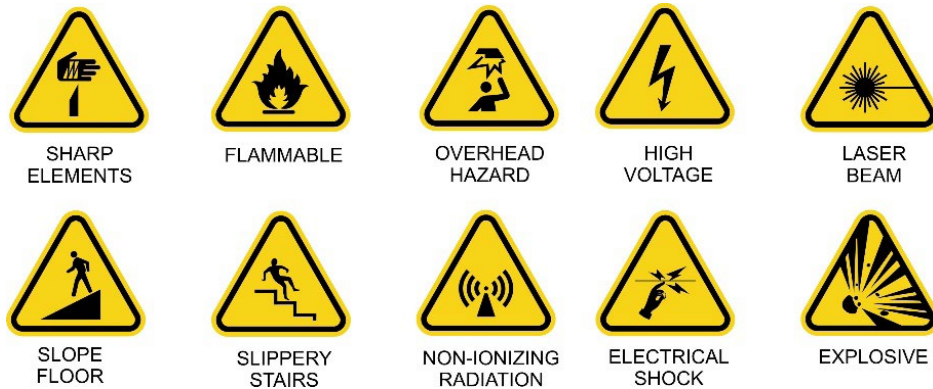
Fig. 3.2.14: Examples of warning signs
