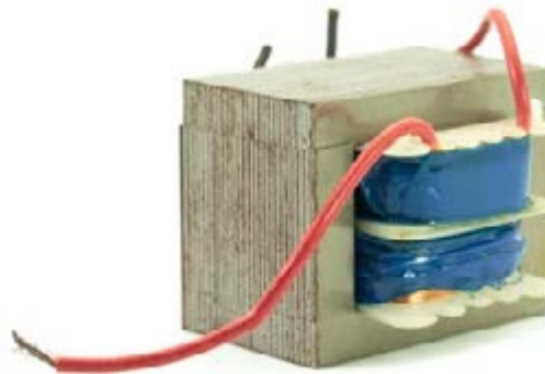
Figure 4.7: A picture of a Transformer
