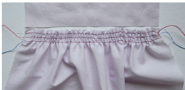
Fig. 7.53: Matching gathered portion with flat piece
