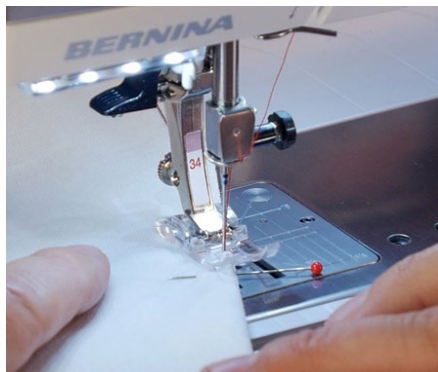
Fig. 7.27: Stitching towards the end of dart
