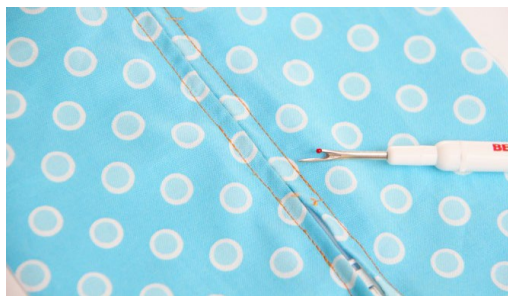
Fig. 7.122: Unpick centre seam
