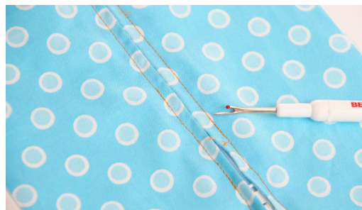
Fig. 7.122: Unpick centre seam
