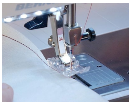
Fig. 7.28: Continue stitching towards the end of dart
