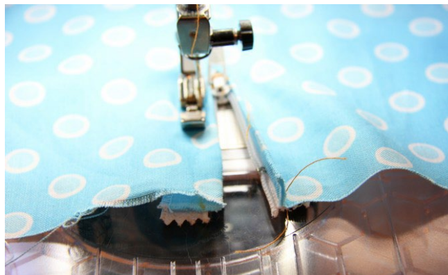
Fig. 7.120: Un-zip the zipper and continue sewing
