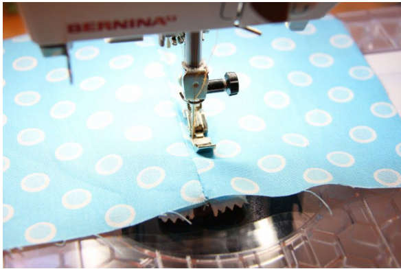
Fig. 7.113: Sew until 5cm to the end
