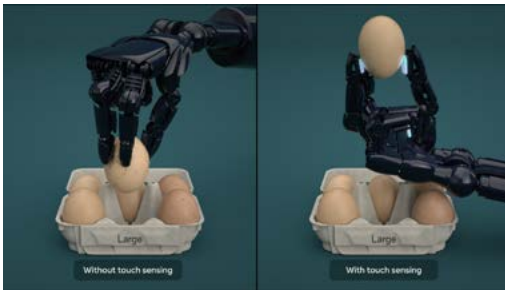
Fig. 3.5: Robotic hand using touch sensing to pick up an egg.
