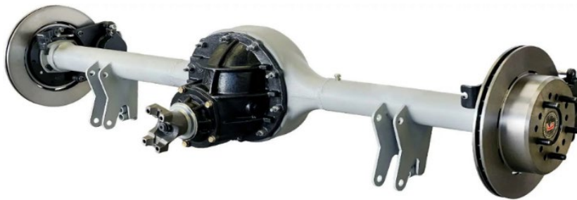
Fig. 4.2.11: A live rear axle
