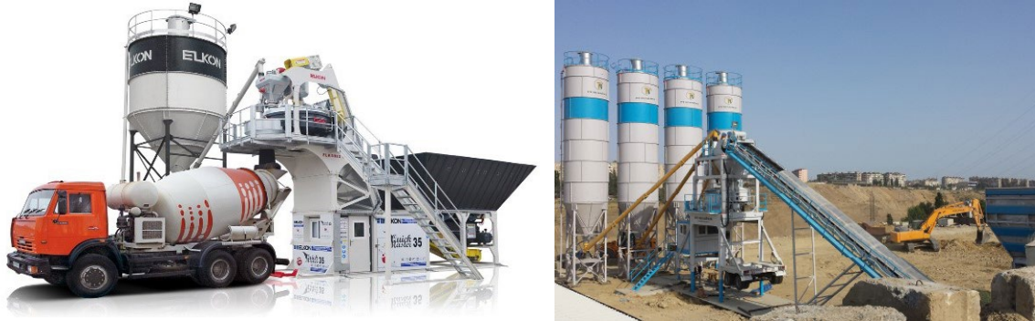
Figure 6.1.3: Batching plants for concrete mixing
