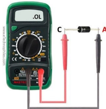
Figure 6.3.3: A diode being tested in reverse-bias using the diode mode in a digital multimeter
