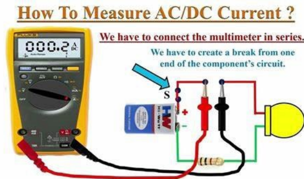
Figure 6.3.5: A multimeter connected as a milliammeter or (Ammeter) to measure current in a test circuit
