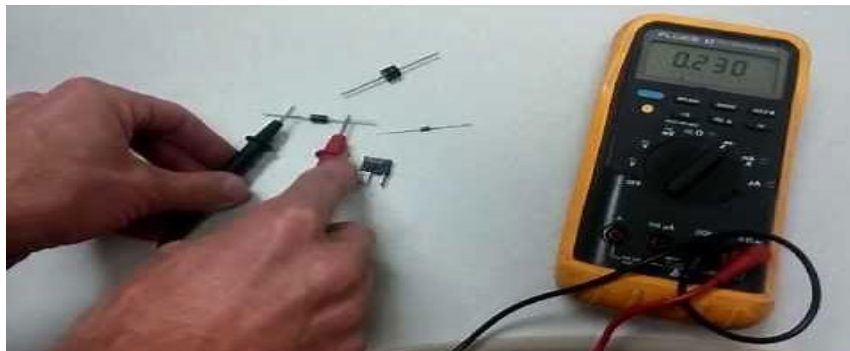
Figure 6.3.2: A technician using a multimeter to test a diode.
