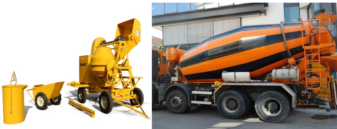
Figure 6.1.6: Concrete Mixers at site. Figure 6.1.7: Mobile Concrete Mixer
