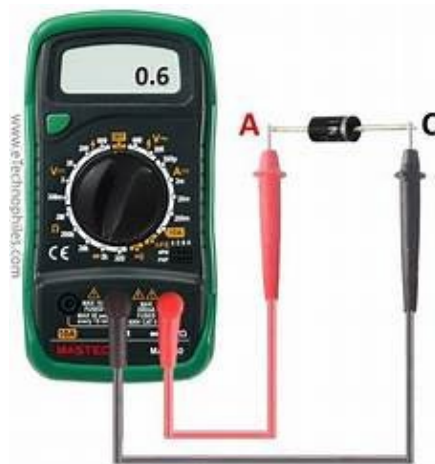
Figure 6.3.1: Diode being tested in forward-bias mode using digital multimeter
