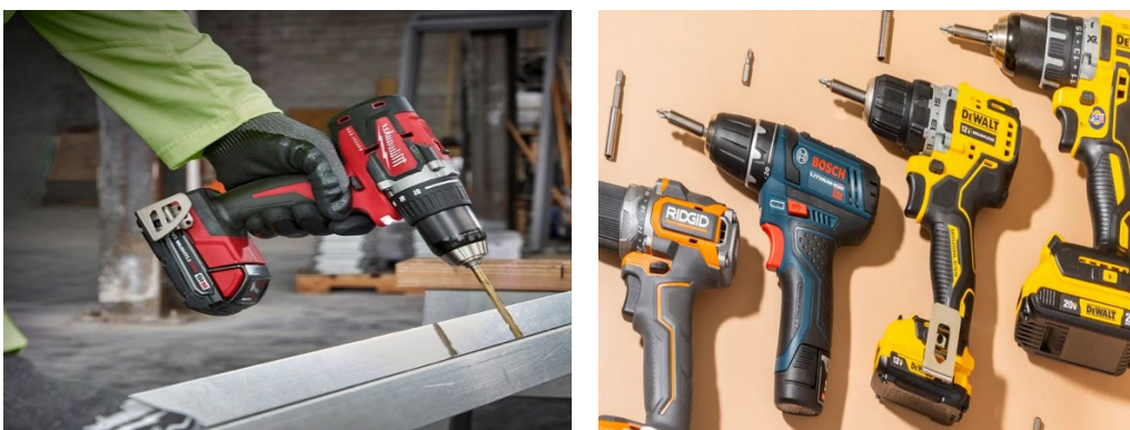
Figure 6.1.4: Power drills used at construction sites
