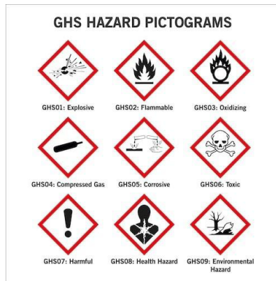
Figure 7.7: Globally Harmonised System (GHS) Hazard Pictogrammes
