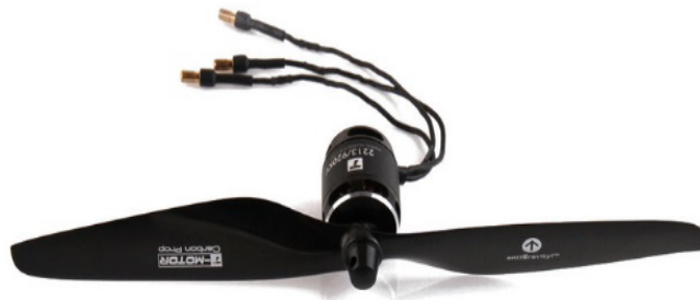
Figure 5.11: A propeller mounted on a brushless motor
