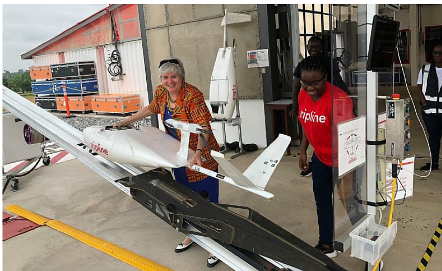
Figure 5.23: UAV catapult launch by Zipline
