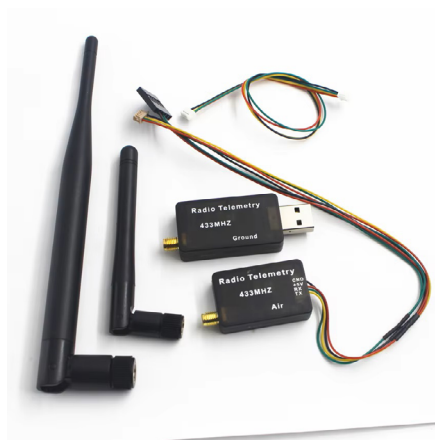
Figure 5.19: Air and ground Telemetry module
