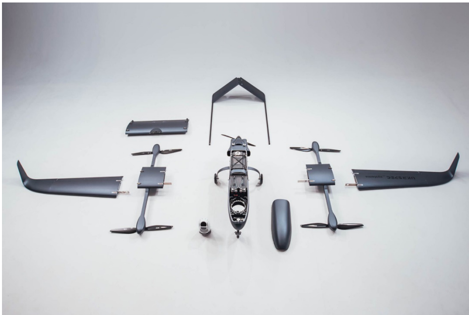
Figure 5.6: Picture of a disassembled airframe
