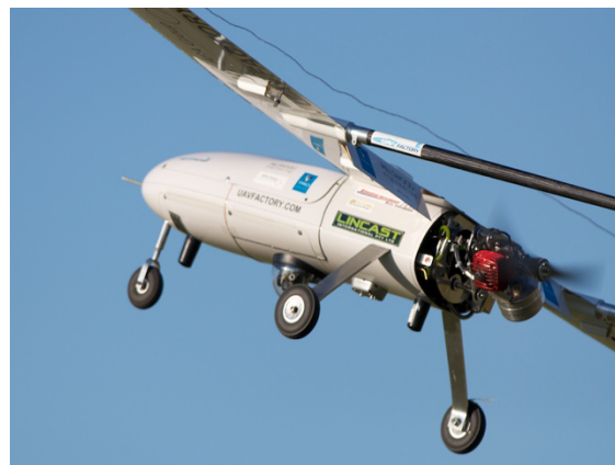
Figure 5.13: A UAV with gas engine mounted in front
