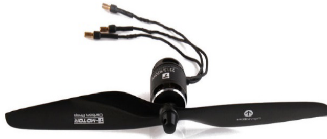
Figure 5.11: A propeller mounted on a brushless motor
