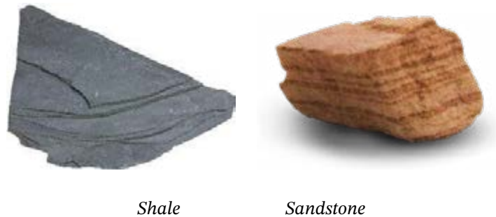
Fig. 7.6: Some examples of mechanically formed sedimentary rocks
