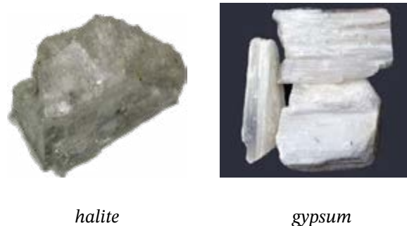
Fig. 7.8: Some examples of chemically formed sedimentary rocks
