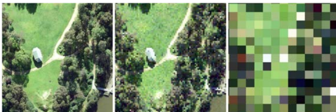
Fig. 9.2: Different resolutions (cell size) of the same raster image
