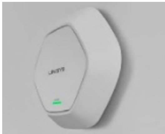
Figure 4.9: A Wireless Access Point (WAP)
