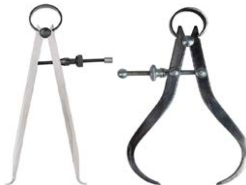
Fig. 5.4: (a) Inside calliper and (b) Outside calliper)
