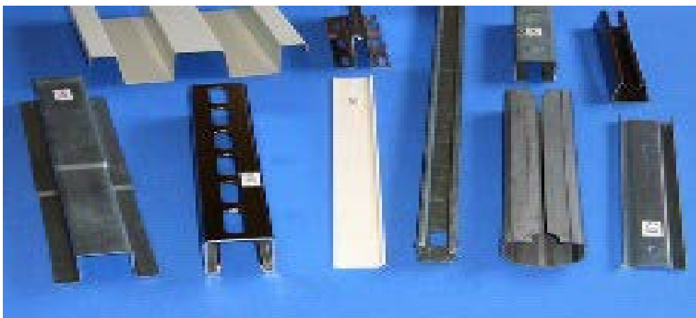
Fig. 6.2: Some products produced by the metal rolling process
