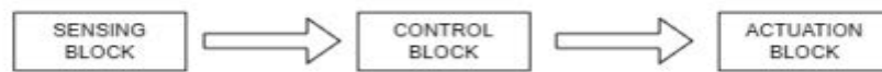
Fig. 4.10 shows the block diagram representation of the robotic system with appropriate labels for each block and arrows indicating signal flow between the blocks.
