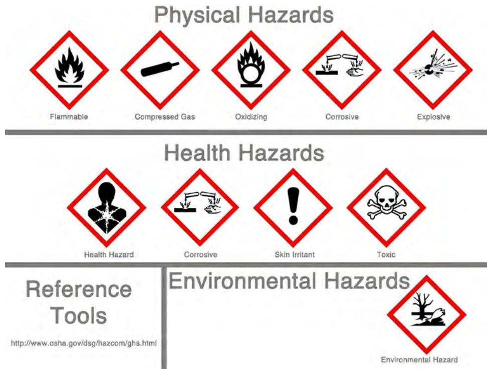
Fig. 8.5: Some examples of health hazards
