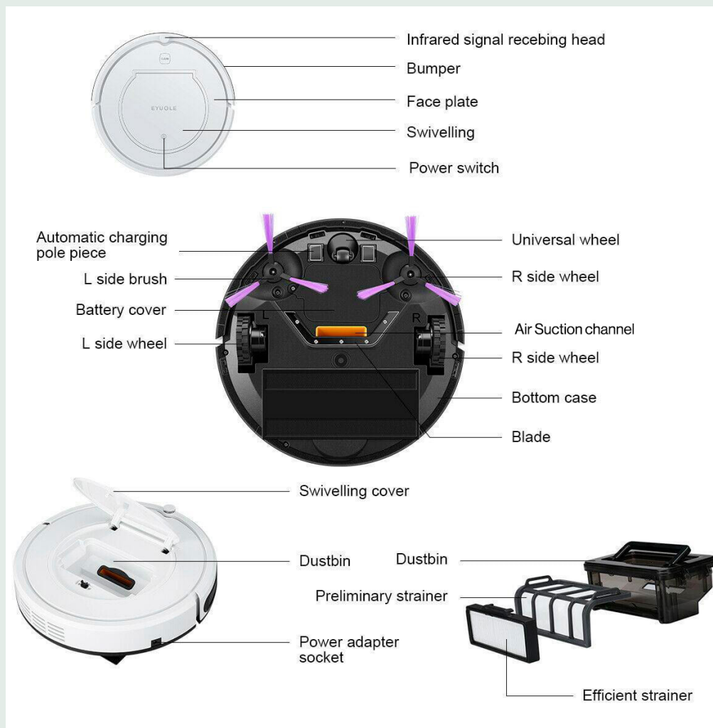
Fig. 2.4 Subsystems of a robotic vacuum cleaner ().
