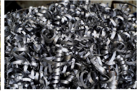
Fig. 16.4: Metal shaving from lathing
