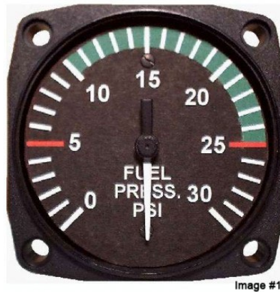
Figure 80: Fuel Pressure Gauge
