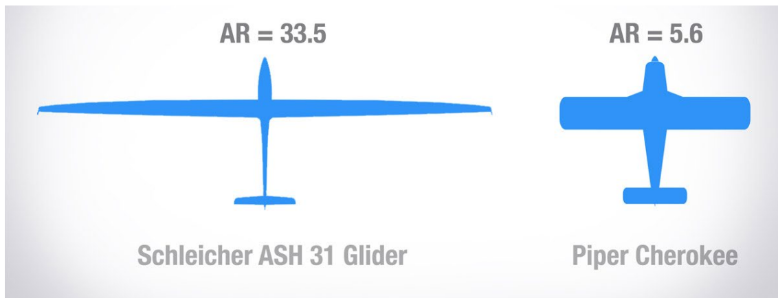
Figure 33: Aircraft with different aspect ratios
