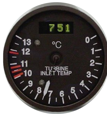
Figure 81: Turbine Inlet Temperature Gauge
