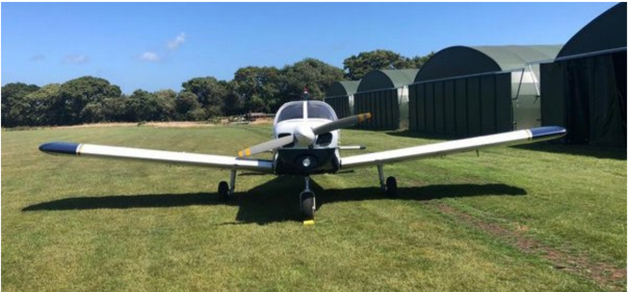
Figure 28: Aeroplane with dihedral wing
