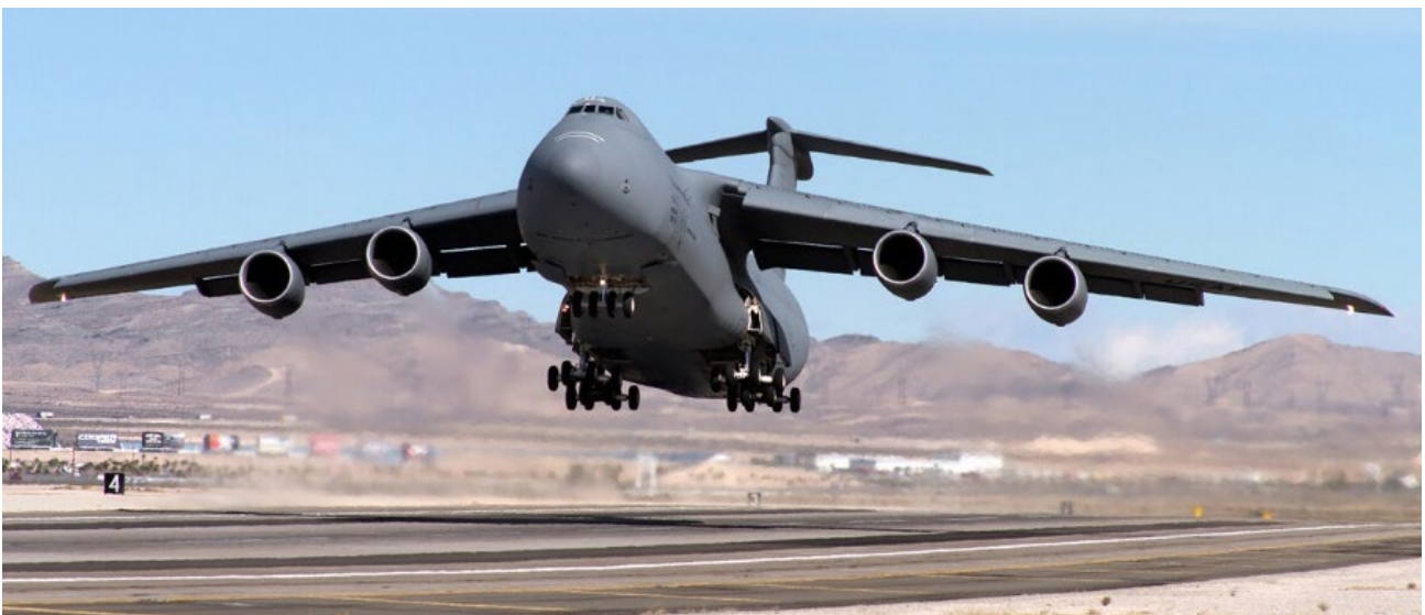
Figure 30: Military cargo aeroplane with anhedral angle
